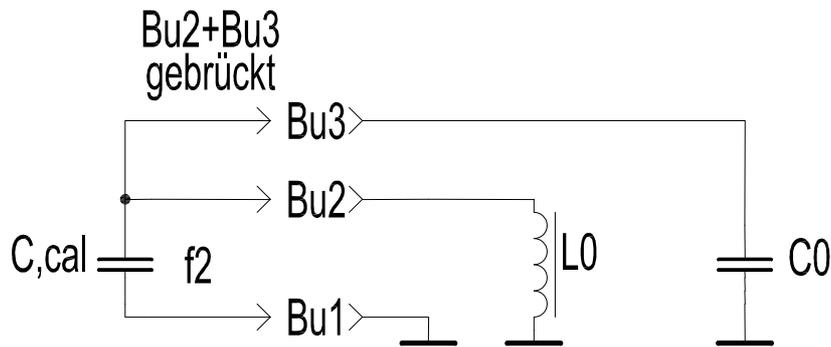
$$\omega_2^2 = \frac{1}{(C_0 + C_{cal})L_0} \quad (2)$$
